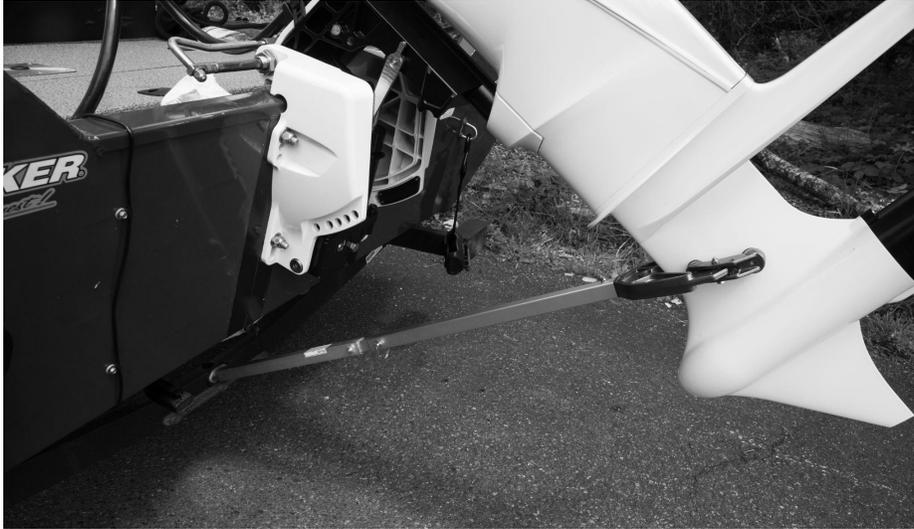
*Figure 8.1 – Outboard Supported by a Transom Saver*
