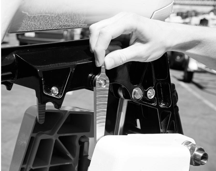
*Figure 5.2 Tilt Lock in the Locked Position*
