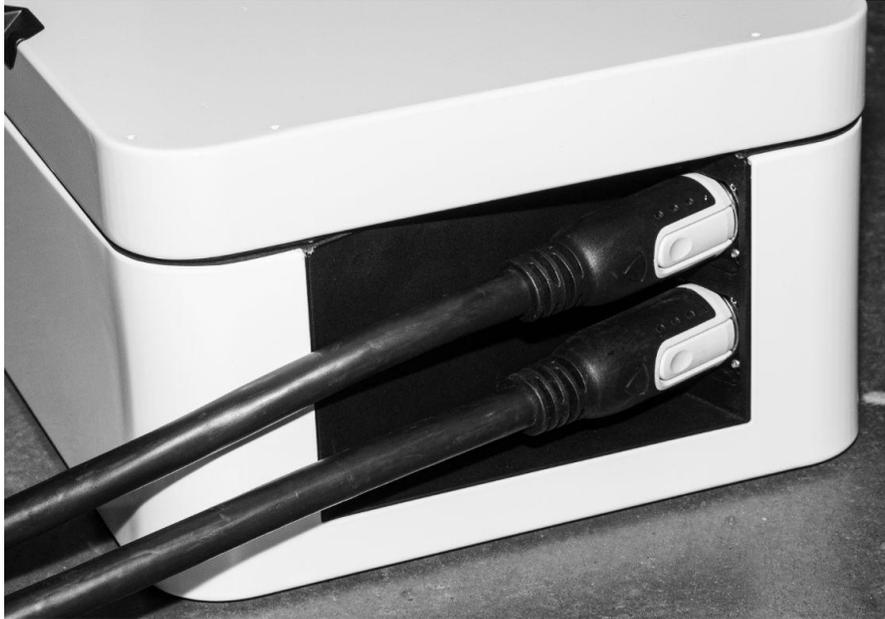
Figure 10.21 – Battery Pack with Power Data Cables Connected
