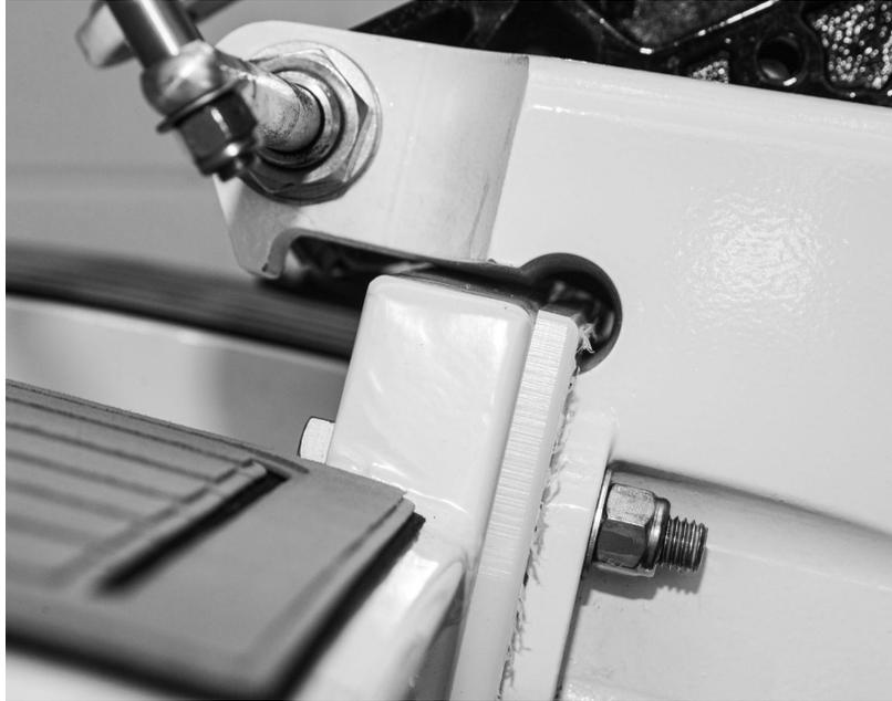
*Figure 10.1 – Appropriate Clearance Between Transom Edge and Inside of Transom Bracket*
