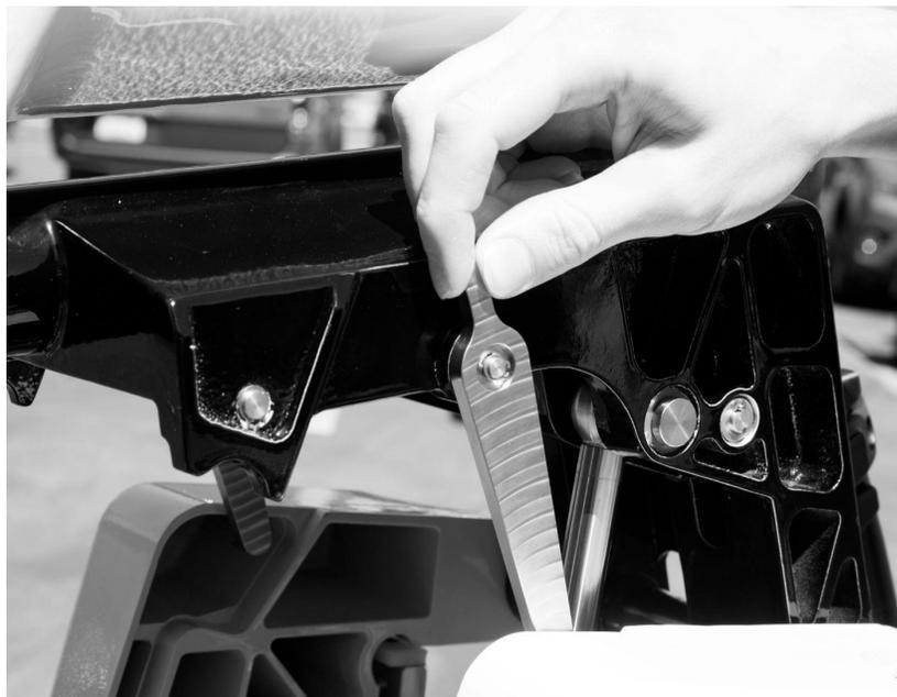
*Figure 4.9 – Tilt Lock in the Ready-to-Lock Position*
