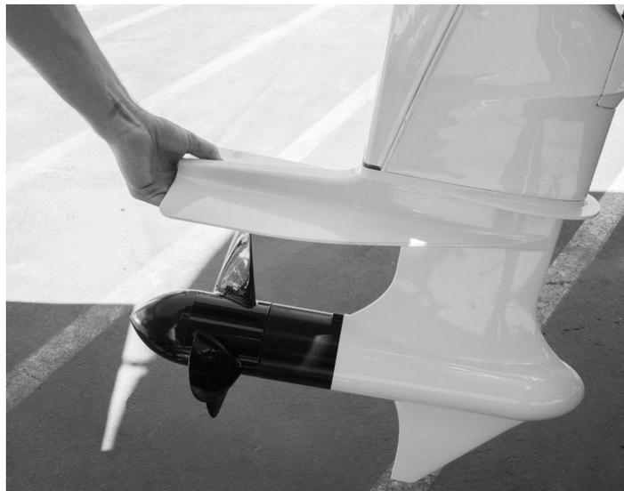
Figure 4.13 – Lifting the Outboard via the Anti-Ventilation Plate
