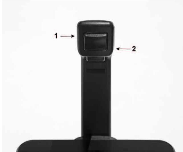
Figure 4.7 – Tilt/Trim Button on the Throttle
