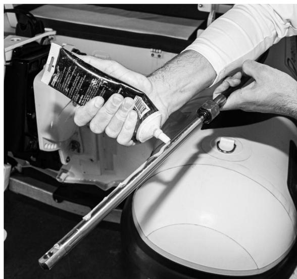
Figure 10.5 – Applying Marine Grease on Steering Cable
