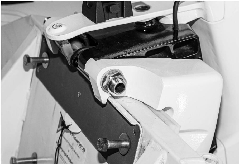
Figure 10.3 – Bolts Aligned in Transom and Outboard
