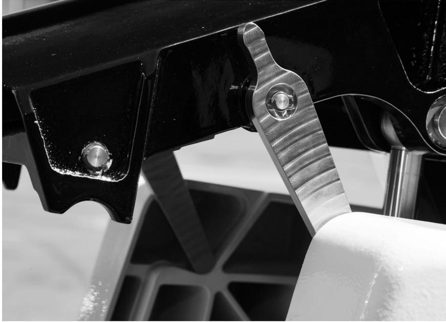
*Figure 9.1 – Tilt Lock in the Locked Position*
