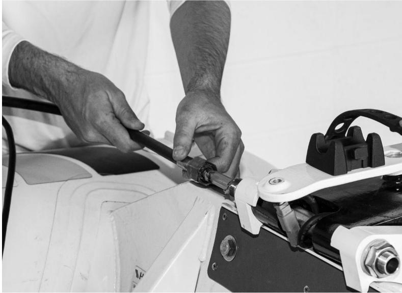
*Figure 10.6 – Inserting the Steering Cable into the Steering Tube*
