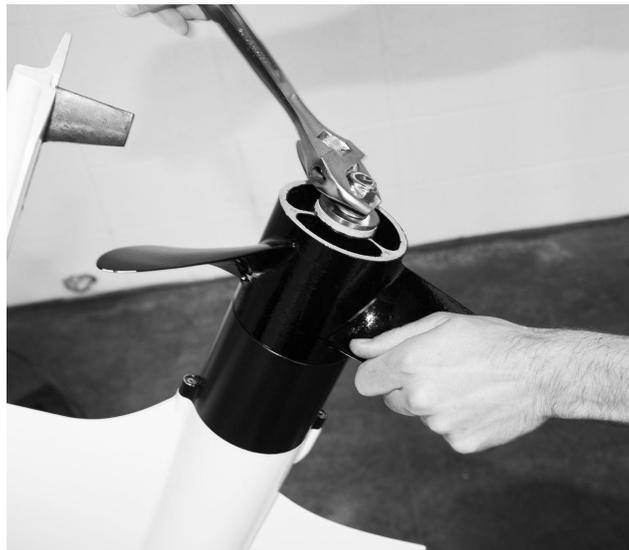
*Figure 10.14 – Tightening Propeller Nut*
