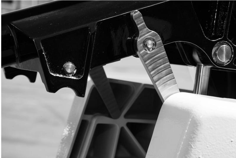
*Figure 4.10 – Tilt Lock Engaged*
