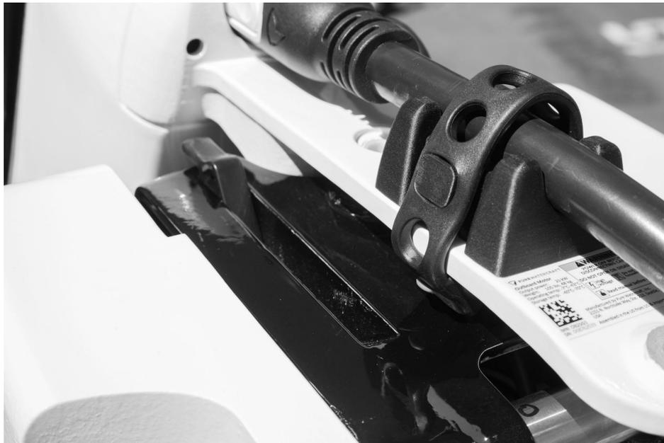
*Figure 5.1 Steering Lock in the Unlocked Position*
