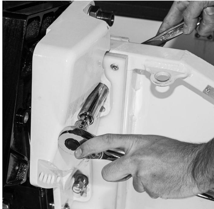
Figure 10.4 – Tightening Bolts with Wrench and Ratchet Extension
