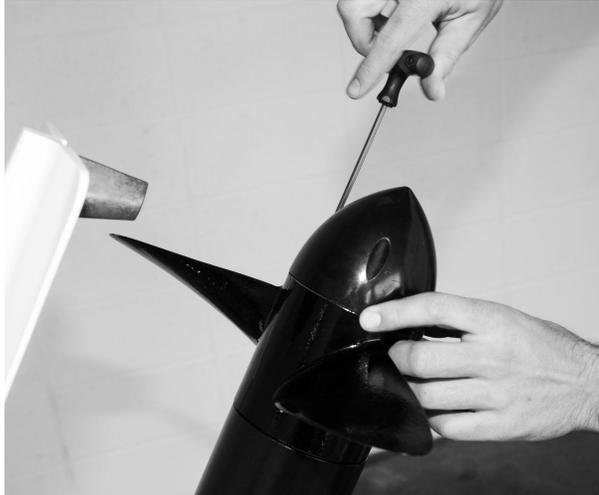
Figure 10.15 – Tightening Tail Cone Fasteners
