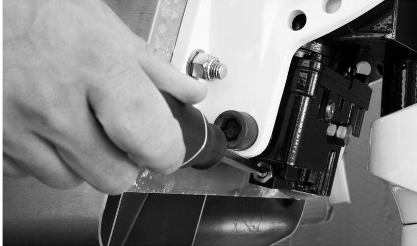
Figure 4.12– Loosening the Release Valve Fastener
