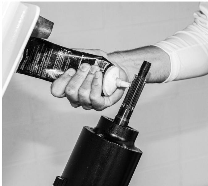
*Figure 10.12 – Apply Marine Grease on Propeller Shaft*
