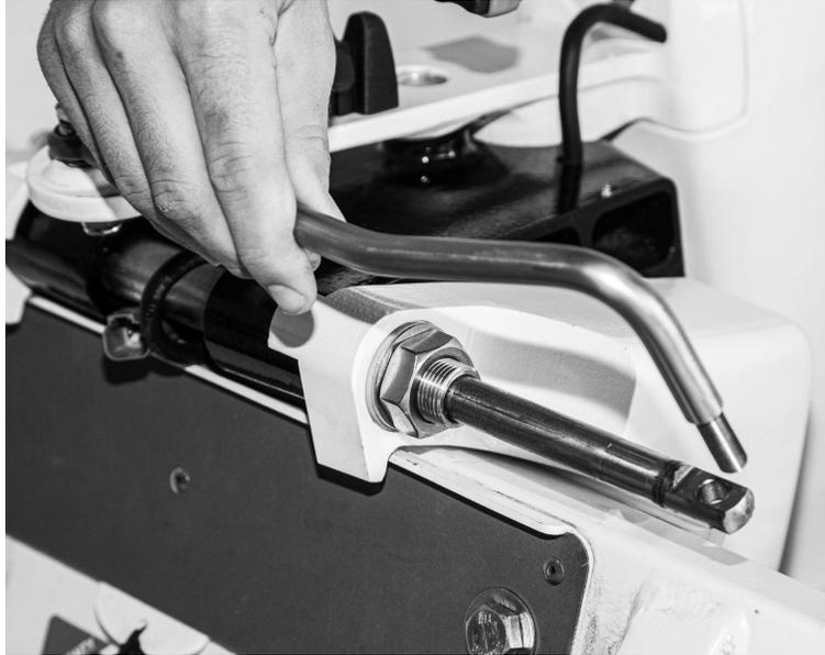
*Figure 10.10 – Insert Steering Linkage on Steering Cable Hole*
